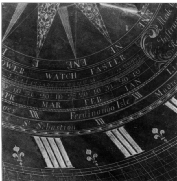
Figure 4: Part of the “Æquation of Natural Days” scale on the Thomas Wright dial at Lacock Abbey (NT), Wiltshire. Note the dates increasing right to left and the maximum of 30 Jan in excess of 14_ minutes.
