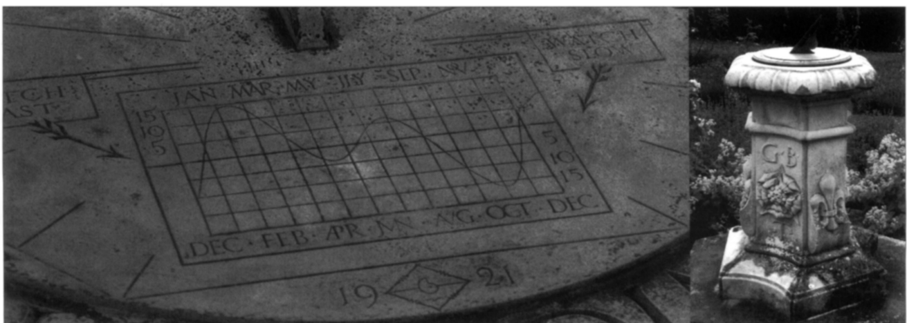
Figure7: The EoT graph on the 1921 dial in the Fellows' garden of Trinity College, Cambridge; possibly the earliest to use this format.
